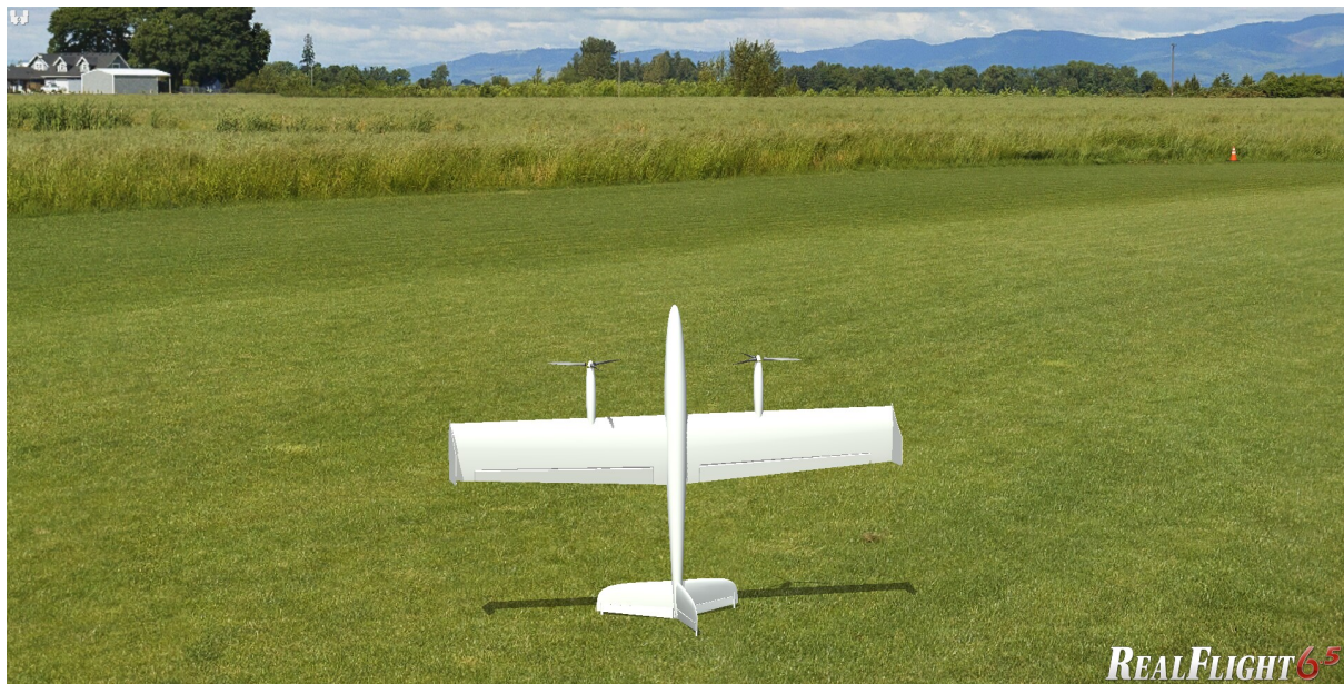
Figure 2. Computer model of the twin-motor tailsitter incorporating the PTVC-M feature. The wing span is 1580 mm.
