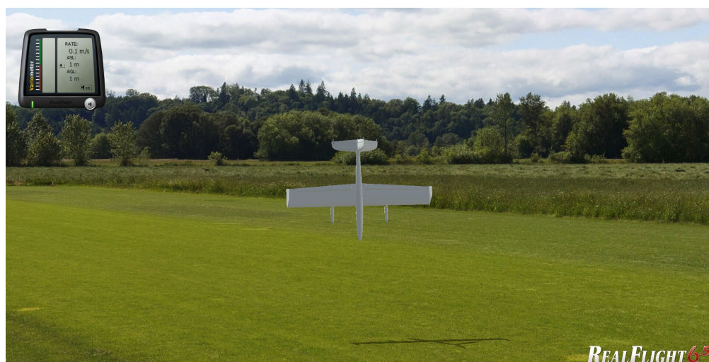
Figure 6. Inverted vertical hover made possible with the surface-free PTVC-M. Variometer shows a climb rate of 0.1 \text{ ms}^{-1} .
