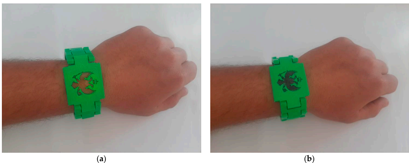
Figure 11. (a) Patient wearing a bracelet without a high temperature. (b) Patient wearing a bracelet with a high temperature.
