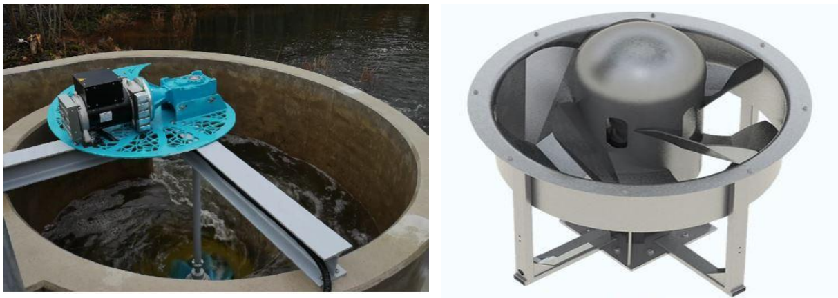
Fig. 4. Vortex turbine - generator system
