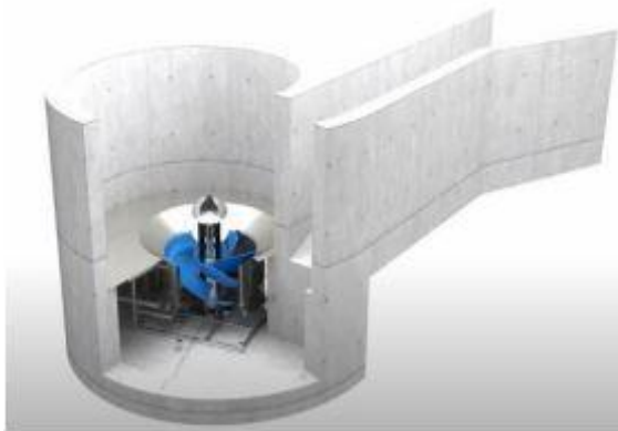
Fig. 1. Installation of a runner in the scroll casing showing the flow path through the turbine
