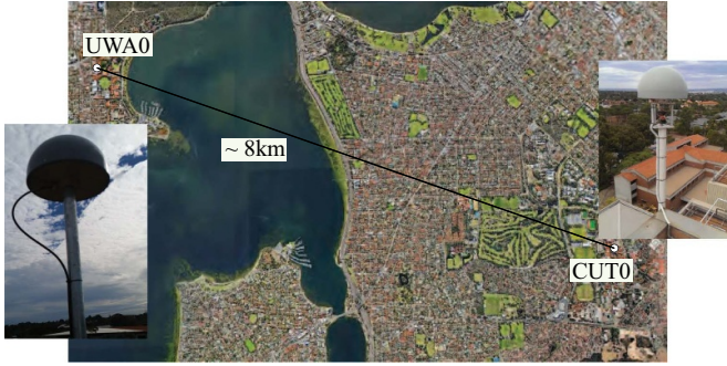
Figure 3. Baseline CUT0–UWA0 located in Perth, Australia: [Left] UWA0 station; [Middle] baseline configuration (Map data @ 2020 Google); [Right] CUT0 station.
