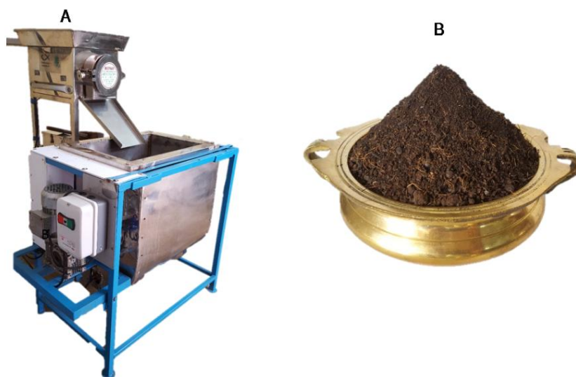
Fig. 1. Waste processing machine (modified model) used for the rapid processing of degradable solid waste to organic fertilizer (A), rapid organic fertilizer produced by thermochemical conversion (B)
