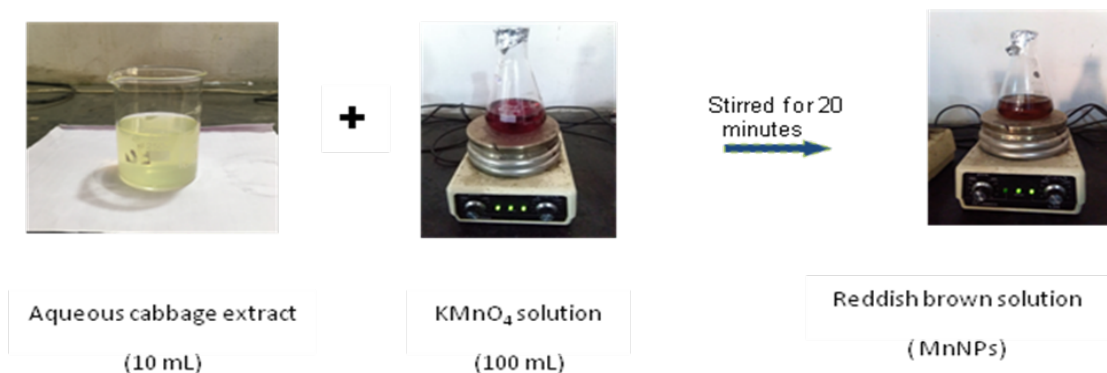
Fig. 1. Biosynthesis of Manganese (Mn) nanoparticles using cabbage leaves extract and 1 mM \text{KMnO}_4 at volume ratio (1:10)
