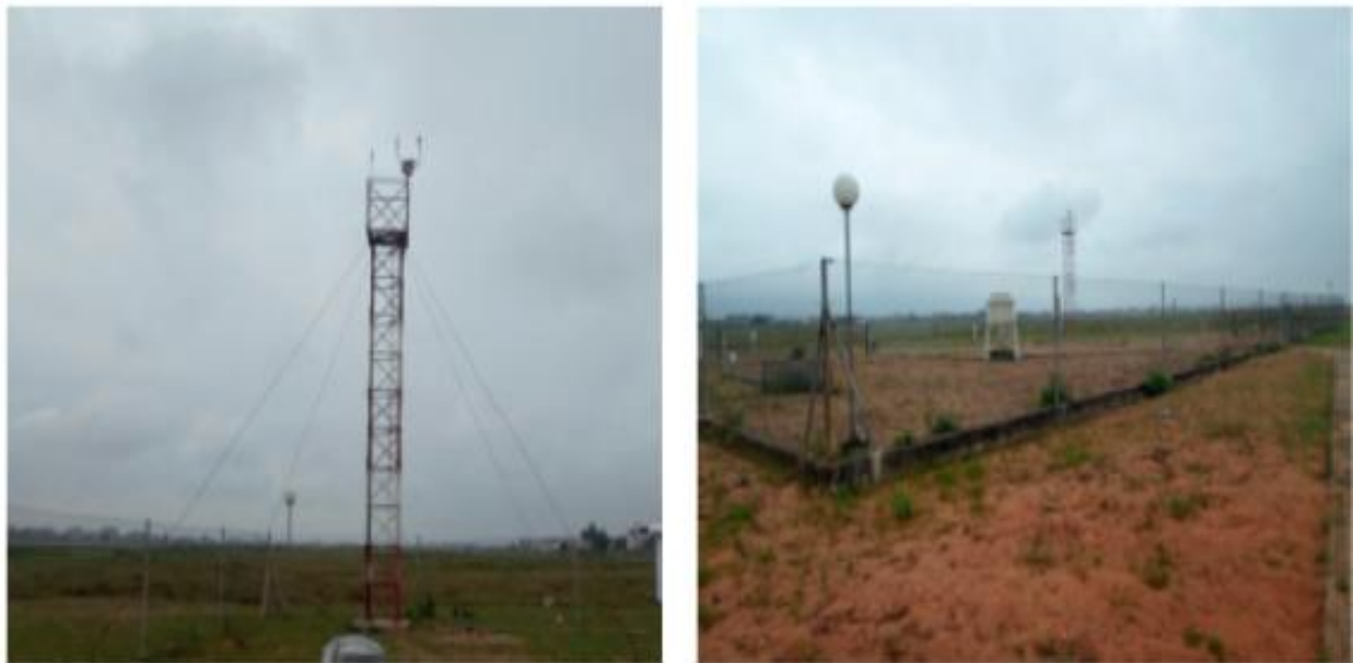
Fig. 1. Experimental site of the Cotonou-Airport meteorological station. Anemometer with cup and wind vane located on a 10 m mast (left panel). Experimentation site (right panel) [12]
