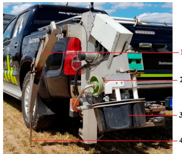
Figure 4. Automatic soil sampling equipment: 1—automatically operated mechanical hand; 2—needle cleaning mechanism; 3—boxes for collecting soil samples; 4—a needle for taking soil samples from a depth of 20–30 cm.
