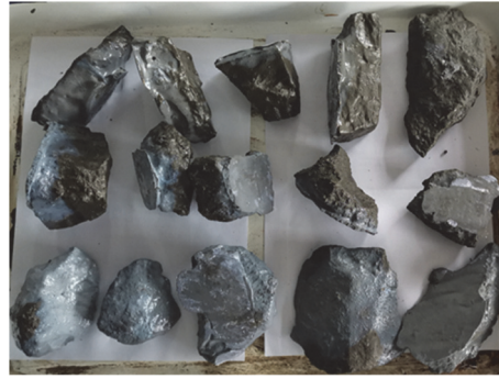
FIGURE 2: Coal gangue specimens coated with pure acrylic emulsion curing agent.
