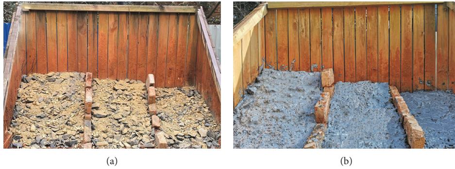
FIGURE 4: (a) Model box A after the laid coal gangue; (b) model box B after spraying the pure acrylic emulsion curing agent.
