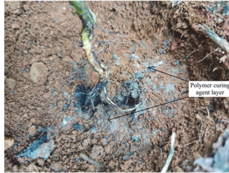
FIGURE 6: Plant roots passing through the curing agent layer.
