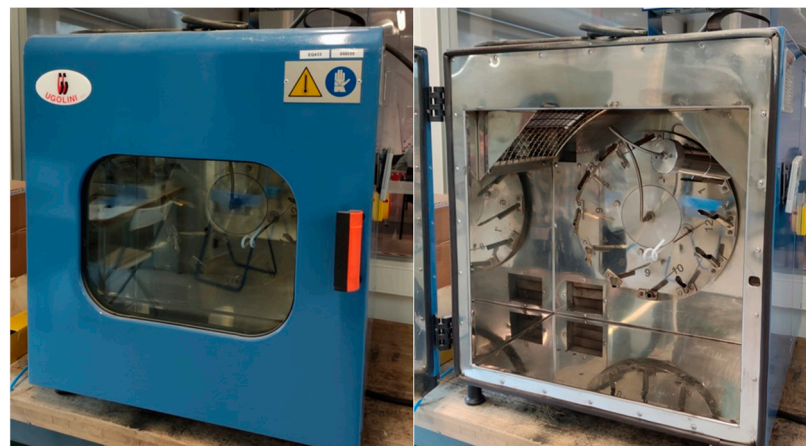
Figure 4. Infrared heat assisted dyeing machine (Redkrome RED P, Ugolini).
