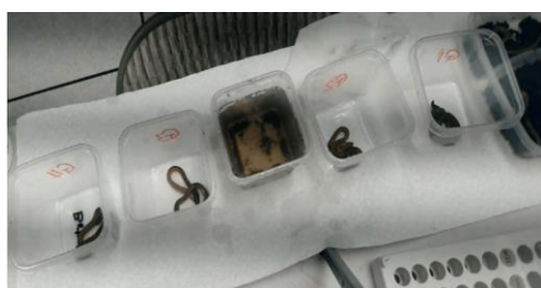
Fig. 9. Shows the procedure of the mass transport study; four nightcrawlers, each inside respective containers, in which toothpaste samples were applied on their skin
