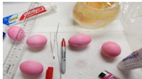
Fig. 7. Presents the procedure of the cleaning capability evaluation with boiled eggs, in which toothpastes were brushed on their surfaces with respective toothpaste samples
