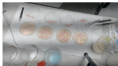
Fig. 8. Represents the procedure of antibacterial strength evaluation, with 4 paper disks soaked in each toothpaste solution - 16 in total - placed on each Petri dish, inoculated with different bacterial strains
