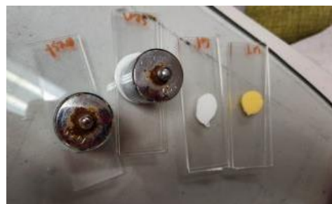
Fig. 5. Shows the procedure of the spreadability evaluation; standard weights are placed on top of toothpaste samples between microscope slides
