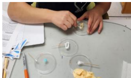
Fig. 4. Represents the scratchiness evaluation, rubbing toothpaste samples onto their respective Petri dishes with sterilized cotton balls
