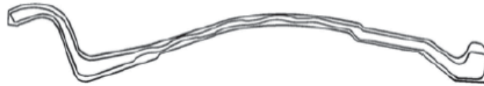
Fig. 8. Finishing and pre-finishing templates when rolling a rim with center wavy part
