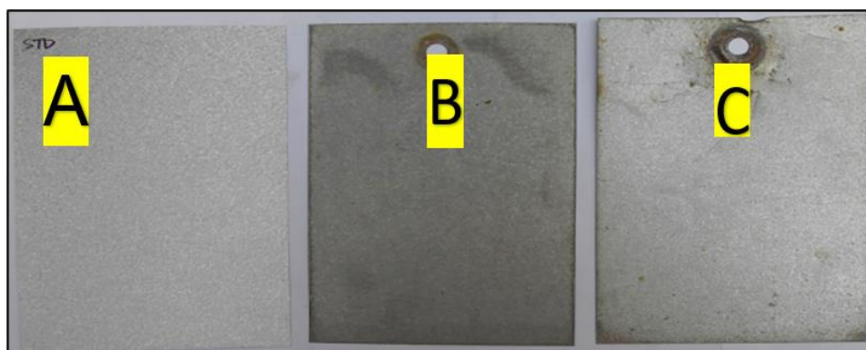
Fig. 5. A photograph showing comparison of corroded specimen (AZ 150) at Mariakani and Diani test sites (A)-control specimen, (B) - Mariakani specimen and (C) - Diani site specimen).
