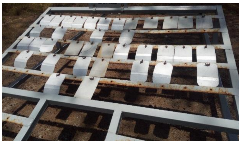
Fig. 2. A set-up for outdoor exposure of 55% Al-Zn metallic coated sheets at Diani site
