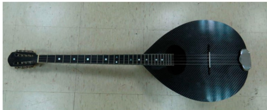
Figure 4. Finalized carbon bouzouki. Reproduced under a Creative Commons Attribution 4.0 International License [23]. Copyright 2023, MDPI.
