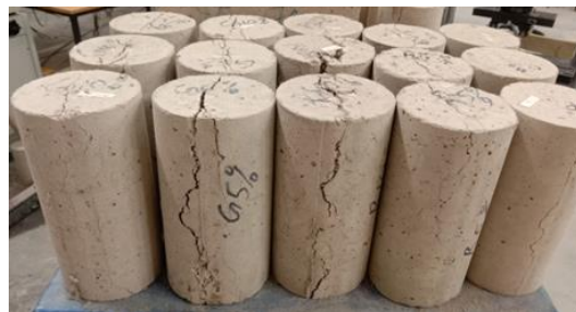
Figure 12. Failure pattern of STS specimens.
