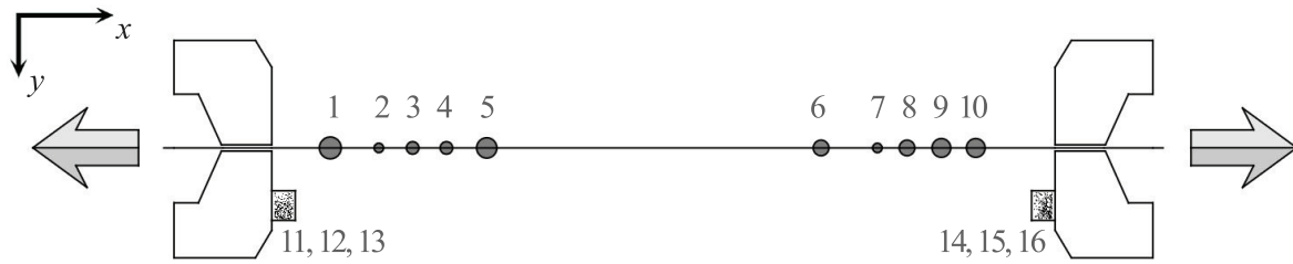
Figure 8. Scheme of pairs of beads evaluated to measure strains directly on the fibre (DSM, facets 1–10) and indirectly on the gripping system (ISM, facets 11–16).
