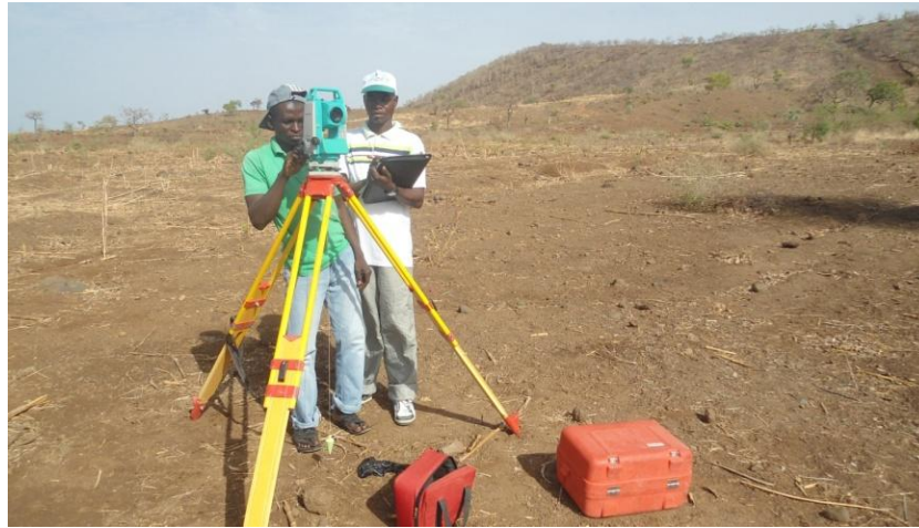
Fig. 1. Sampling at Kumba crater using total station (SOKKIA 630R)
