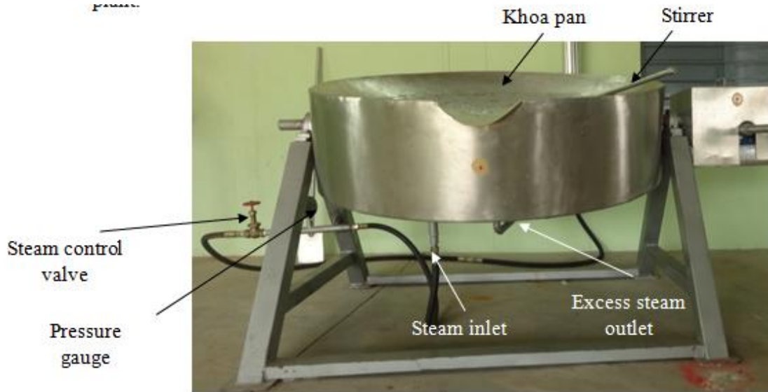
Fig. 3. Steam jacketed khoa pan installed at dairy and food processing pilot plant, CAE, Madakasira
